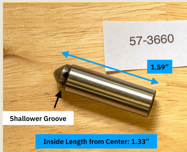
Figure 15: This plunger has a steeper point and a more positive connection with the camplate
