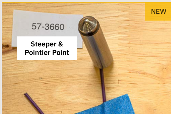
Figure 9: Plunger 57-3660 was new for 1969 and used in 1970
