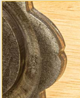
Figure 17: Camplate 57-3650 was used in 1968 and part way through 1969 only—notches between gears were unique to this camplate
