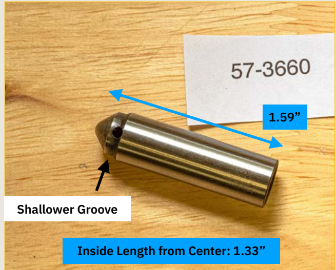
Figures 24: Plunger 57-3660 was first used in 1969 and has a shallower machined groove and a steeper point
