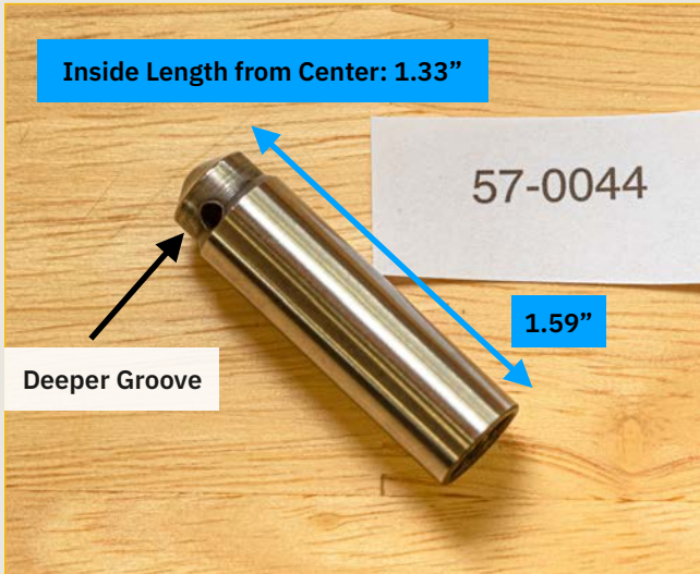
Figures 23: Plunger 57-0044 was used in the '60s through 1968—it has a deeper machined groove and shallower, more rounded point
