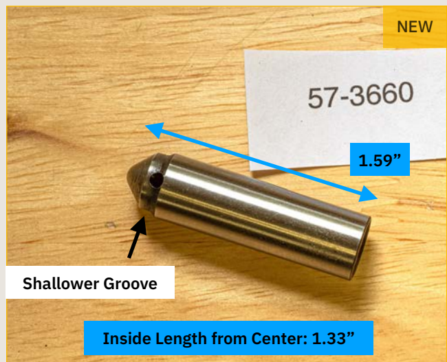
Figure 10: This plunger is the same outside & inside length as the plunger used in 1968
