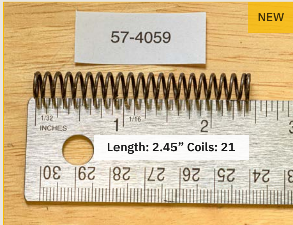
Figure 11: Spring 57-4059 was new for 1970
