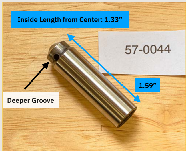
Figure 5: The deeper machined area and shallow tip distinguish this plunger
