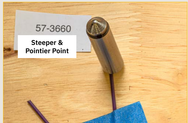
Figures 24: Plunger 57-3660 was first used in 1969 and has a shallower machined groove and a steeper point
