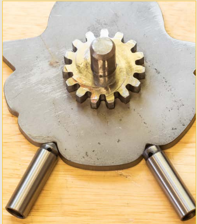
Figure 20: New camplate with new plunger on the left and old plunger on the right; old plunger does not seat well in the gear detent
