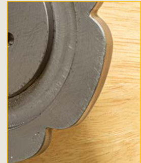
Figure 18: Camplate 57-4055 was new part-way through the 1969 model year; it is larger than its predecessor and does not have notches between the gears
