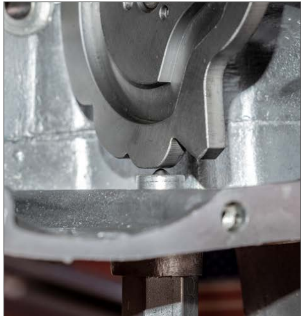
Figure 16: The point at which the camplate is between gear detents is the point at which the spring is at its most compressed state; this is the point of the maximum working load of the spring
