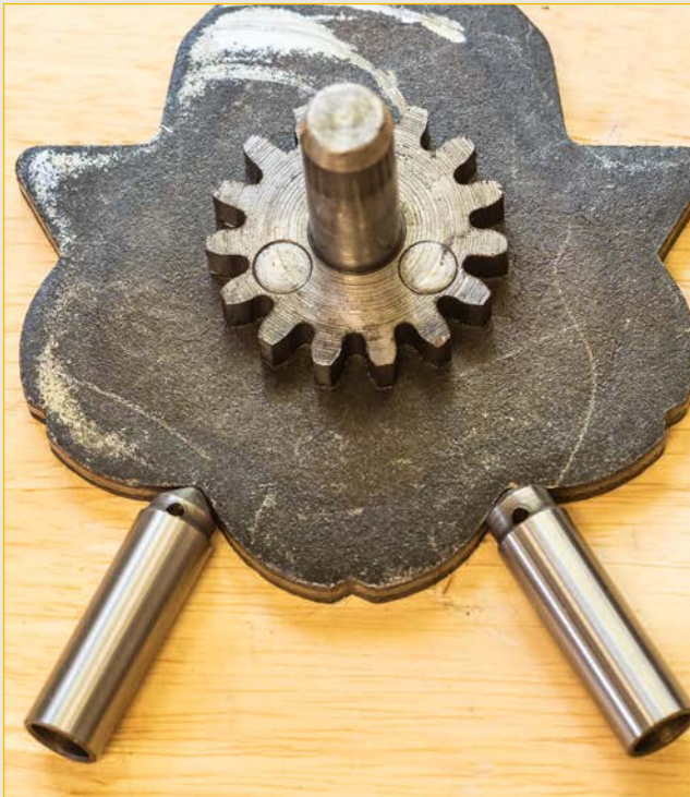
Figure 19: Old camplate with new plunger on the left and old plunger on the right; old plunger fits the gear detent better
