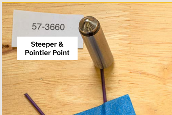
Figure 14: Plunger 57-3660 carries over from 1960
